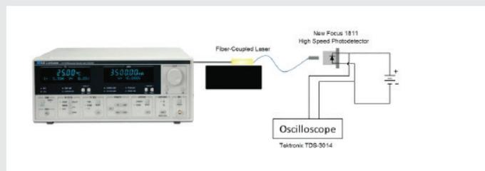
Figure 4: Schematic of transient testing of the LDC-3736 Quantum Cascade Laser Controller
