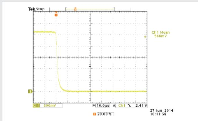
Figure 3: Fast shut down response of the LDC-3736
