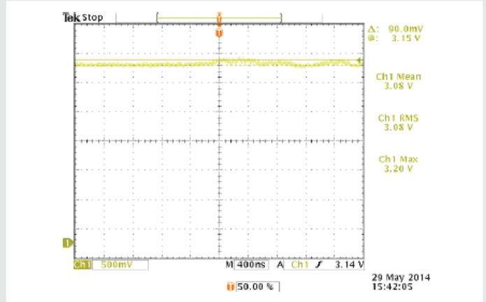
Figure 7: Effect on laser output due to 1 kV power surge event on AC power line
