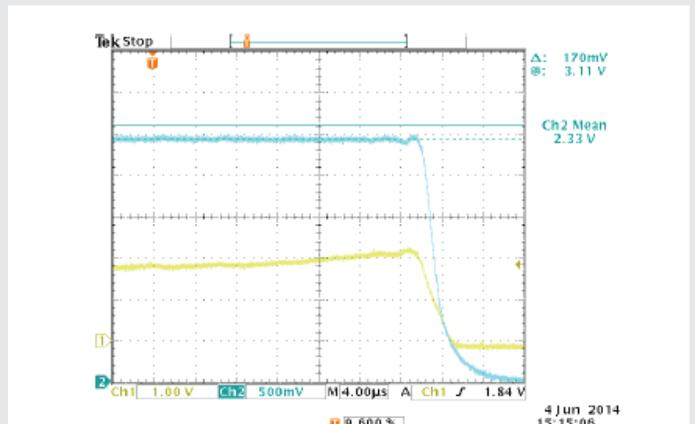
Figure 8: Intermittent contact response of the LDC-3736 with appropriate voltage limit setting
