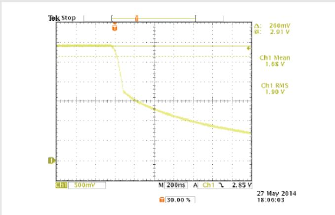
Figure 5: LDC-3736 laser current disabled due to loss of power or brown out
