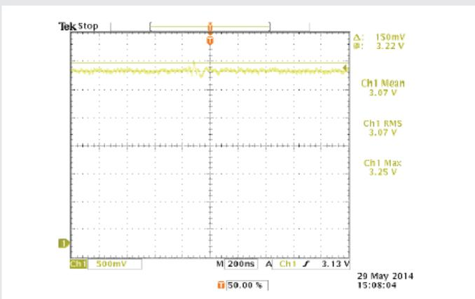
Figure 6: Effect on laser output due to 1 kV EFT event on AC power line
