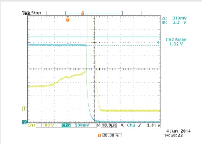
Figure 9: Intermittent contact response of the LDC-3736 with improper voltage limit setting
