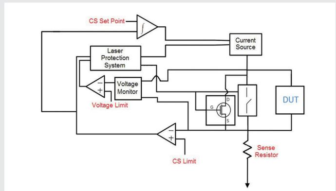
Figure 1- Schematic diagram of the LDC-3736 laser protection system circuitry
